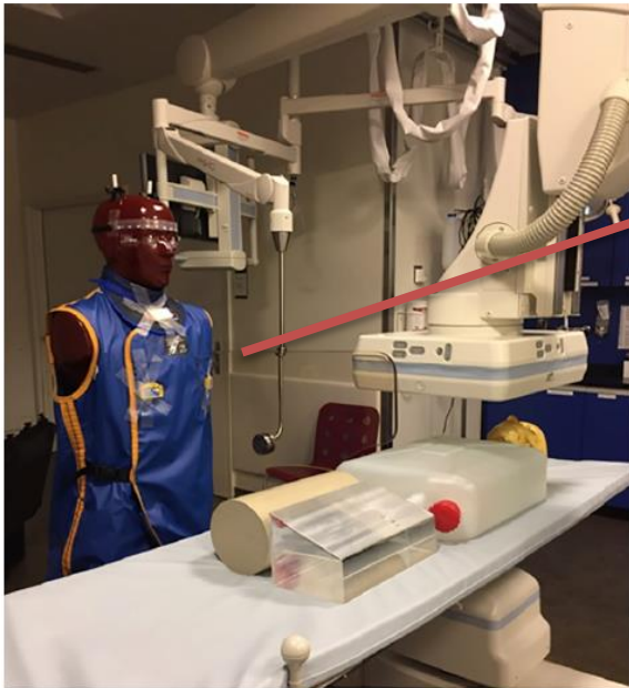
Fig. 5. Position of the phantoms and dosimeters during the measurements in the radiological room.
