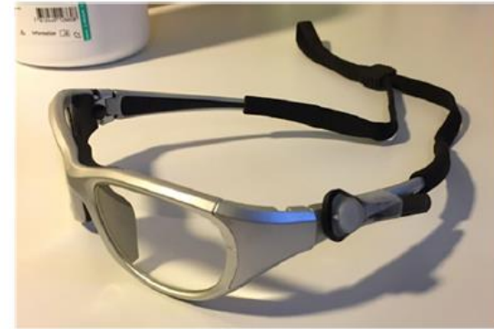
Fig. 6. Typical position of the Dosiris dosimeter taped on protective glasses.
